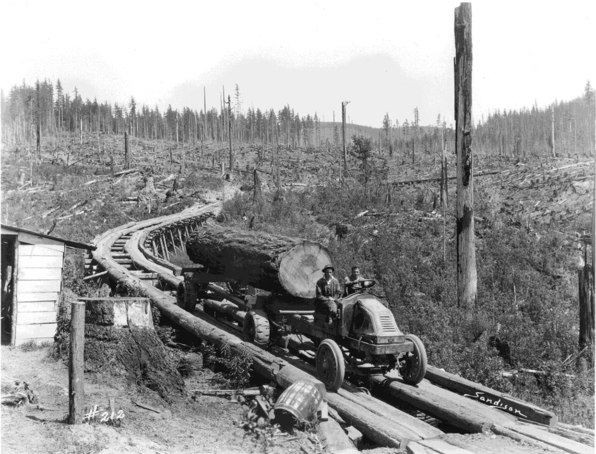
A Kelly-Springfield logging truck hauls a large fir log along a track-like wooden logging road. Behind the truck are acres of cutover land, ca. 1925. Photograph by J. Wilbur Sandison, courtesy of the PEMCO Webster and Stevens Collection, Museum of History and Industry, Seattle 1983.10.3675.10
